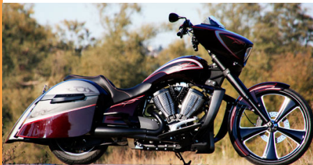
Customizing idea: Kodlin 2011 Cross Country with custom 26 inch front fender, wheels, fenderbags and stretched and lowered gas tank.
