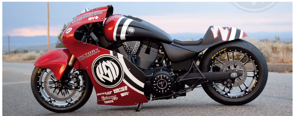
Project 200 - In 2010, Roland Sands took a 2011 steel frame and had Lloydz build a Big Bore motor with Garrett Turbo and intercooler. Belt was tossed in favour of a chain. The result dyno-ed out at 214.29 horsepower with 243.54 pound feet of torque.
